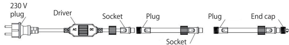
To expand the LED strip, connect the plug and socket together. Please make sure that the union nut and the end cap are screwed correctly and tightly!
