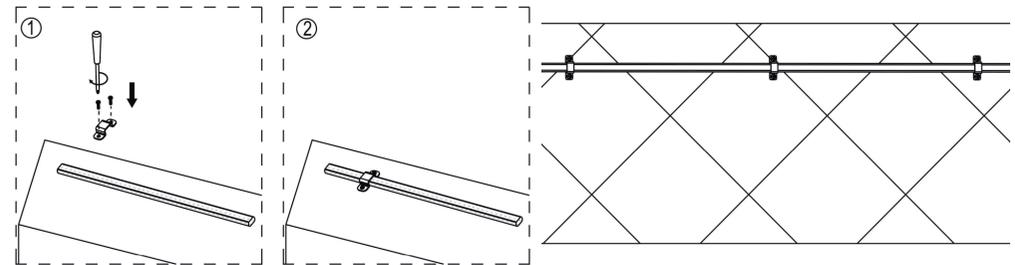
Use suitable clamps or holders for permanent attachment. Do not use thin wire or similar to attach it, as this could damage the plastic coating. In the case of longer or permanent installation, the LED stripe must be fixed vibration-free in order to prevent line breaks.
